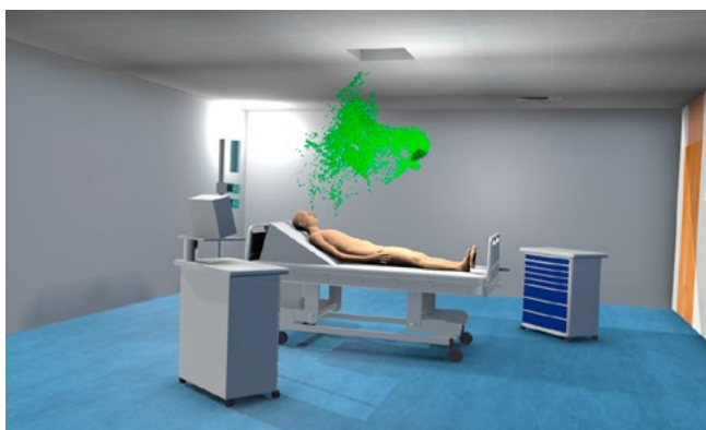
Figure 7. Airflow within a hospital room can be evaluated for transmission potential of airborne pathogens. Redesign to minimize possible transmission can be performed rapidly and safely. Hôpital Saint-Louis airflow simulation illustrate such case.
